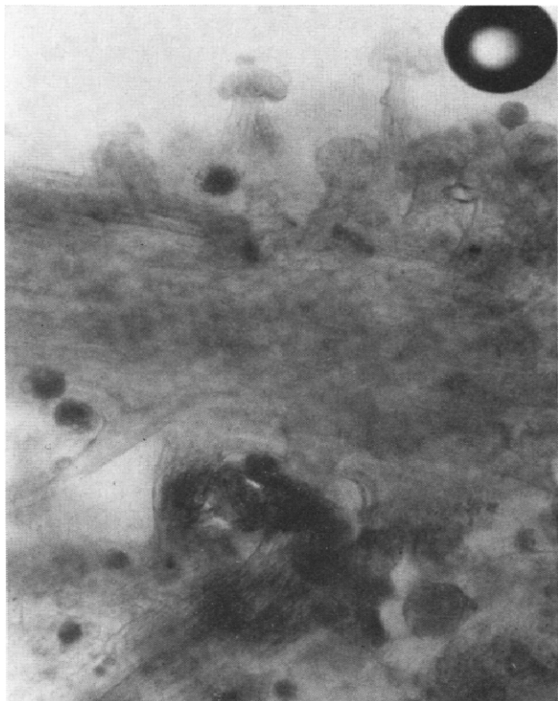
Fig. 3. Microscopic appearance of plant material shown in Fig. 2, 20 sec after treatment with Fast Blue B chromogenic reagent. Note that the cannabinoid-containing tissues have rapidly acquired pink to red colors (shown as darker shades in black and white).
